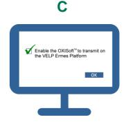
Flag the box "Enable OXISoft™ to transmit on the ERMES platform". Press OK. Flag which Oxitest (OXISoft™ manages up to 4 units) you want to enable.
